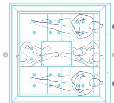
The Venus spa has **4 seats (2/2)**. Manufactured in one piece in **satin-finish AISI-316L stainless steel** with a thickness of 2 mm.
