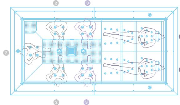
The Zeus spa has **7 seats (5/2)**. Manufactured in one piece in **satin-finish AISI-316L stainless steel** with a thickness of 2 mm.
